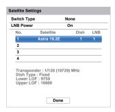
Once you have selected a satellite, you can change further settings under **Dish** and **LNB**. Press **OK** and **◄**/▶ to select **Dish** or **LNB** and press **OK**.
